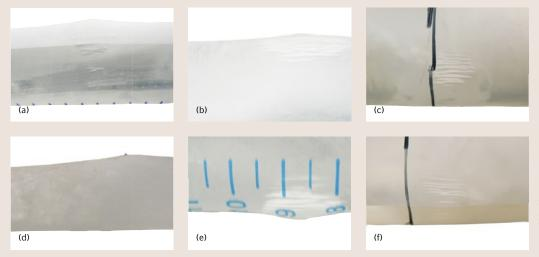
Figure 1: Stress lines and bulging (a-f) caused by increased pressure from liquid expansion in 15 mL and 50 mL conical tubes stored in various storage boxes from other manufacturers without temperature compensation vents.
