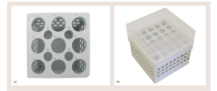
Figure 3: Eppendorf Storage Boxes for (a) 50 mL conical and (b) 15 mL conical tubes, with temperature compensation vents throughout the base of the boxes, designed to provide a homogeneous freezing process.
