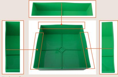
Figure 8: Shape deformities in storage boxes from various manufacturers after cleaning and/or autoclaving. The dividers no longer fit properly into the base of storage boxes from Manufacturers E and F.
