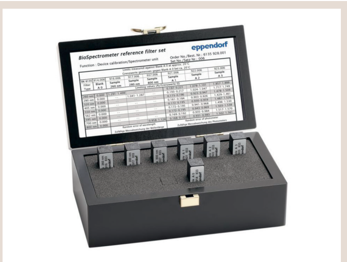
Figure 1: Eppendorf reference filter set for checking photometric and wavelength accuracy of the Eppendorf BioSpectrometers basic and kinetic.
